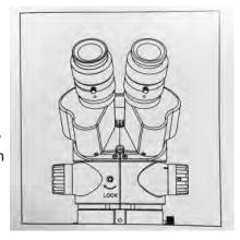
While looking through microscope, move viewing head up or down on post until object can be seen in approximate focus. Tighten focusing holder locking knob. Position the support collar under the focusing block and tighten locking knob on support collar. It is not necessary to make
