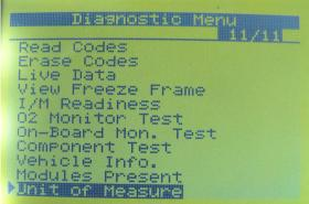
Unit of Measure 2/2 Enslish Metric **Note:** When you finish the diagnostics, in the Diganostic Menu, press NO button, then press YES to exist OBDII Test.
