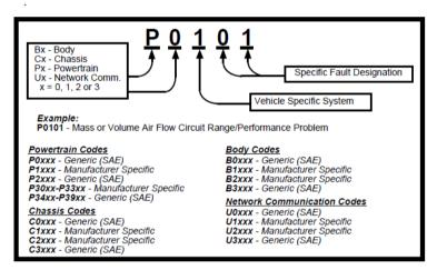
Within each category (Powertrain, Chassis, Body and Network) of DTCs there are assigned ranges for different vehicle systems.
