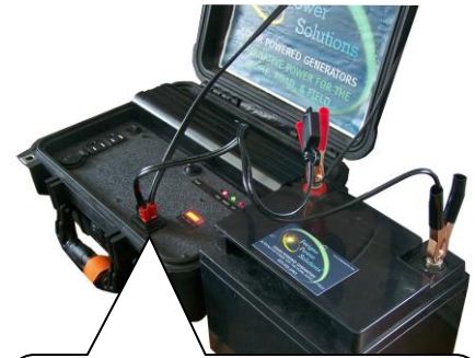
Image shows 44Ah AUX battery & MPI cable connected to a 201 kit multiport with a 45W panel also connected to the Solar In (panel not in frame).
