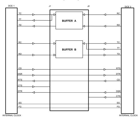
Note: The buffers introduce transmission delay into the data paths between the DCEs. The control signals, however, are not buffered and are just wired through, as shown. This should be considered when using the 3004-ECB in applications where the data and control signals must have the same delay.
