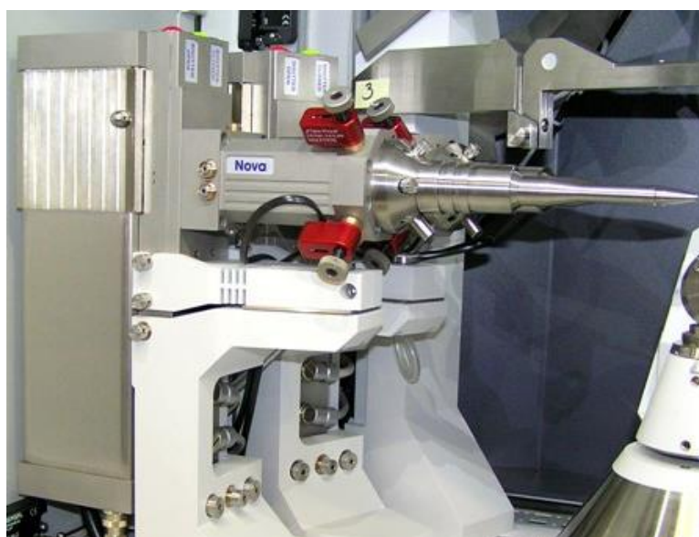
Figure 11 Microfocus X-ray source mounted on SuperNova diffractometer
