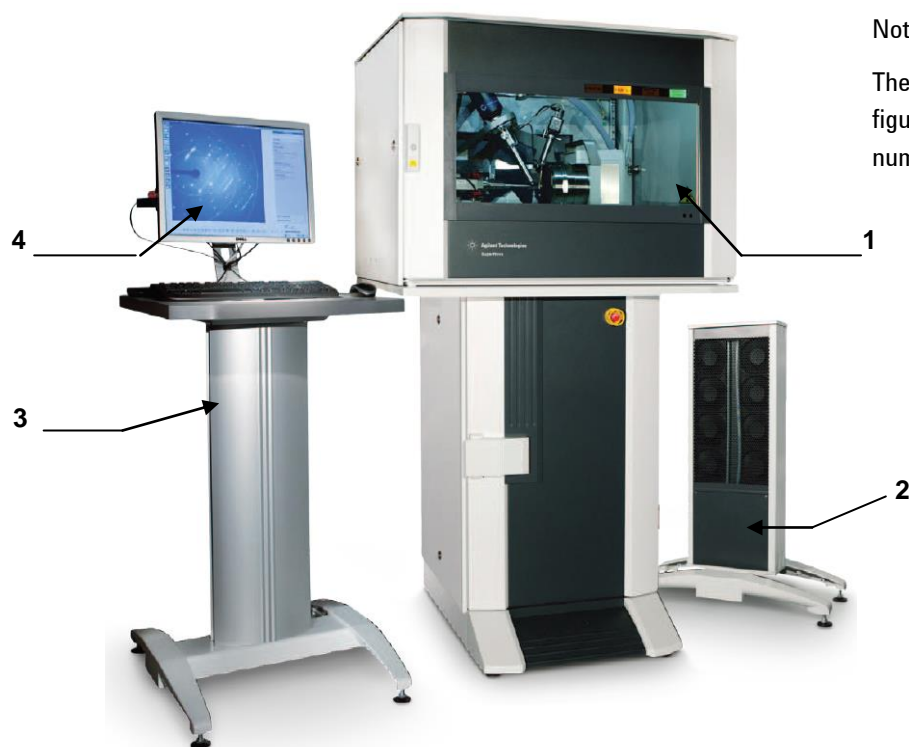
Figure 1 Components of a typical SuperNova system
