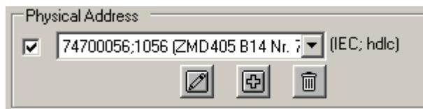
The physical device addresses for the required meter can be selected in the "Physical Address" selection box, provided the check box is marked.
