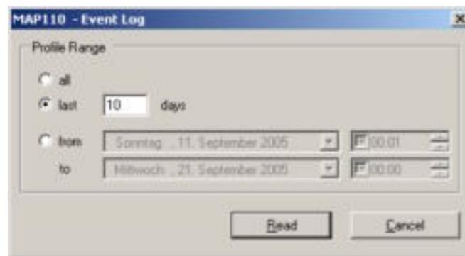
The event log data read out are shown as a table in the display window. With readout under dlms the table contains the date and time, EDIS status word, event number and register statuses for every event. An explanatory text is displayed by placing the mouse pointer on a column heading or a cell. In the case of a coded EDIS status word, this is directly decoded and all individual events are displayed (e.g. the EDIS status word 00880080 contains the individual events 8, 20 and 24).
