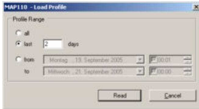
The load profile data read out are shown as a table in the display window. With readout by dlms the table contains the date and time-of-day, EDIS status word and the register statuses recorded for every integrating period. An explanatory text is displayed by positioning the mouse pointer on a column heading or cell. For example the significance of the coded EDIS status word (see also table in chapter 7.1.3 "Read Commands for Event Logs") are decoded directly and all individual events displayed.
