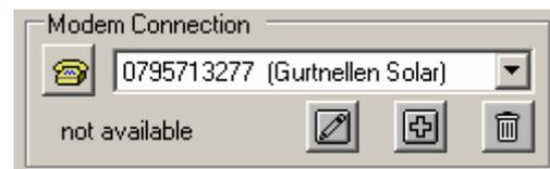
The call number of the required modem can be selected in the "Modem Connection" selection box, if a modem is selected as interface in the communication settings. Otherwise the area is deactivated, i.e. set for a local connection.
