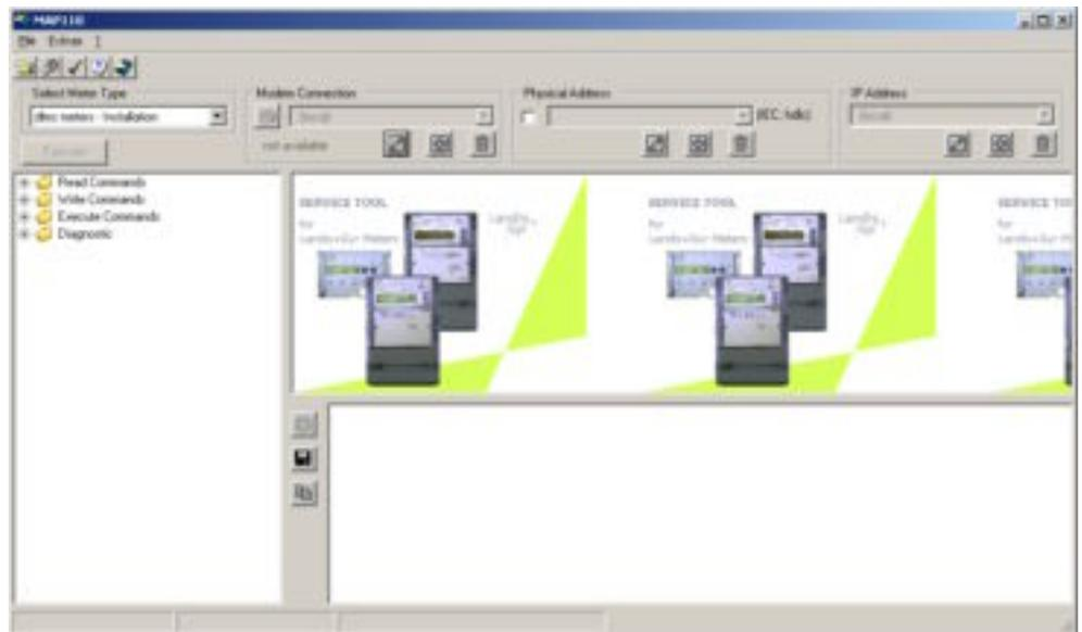
3. In the selection box "Select Meter Type" select the meter type "dlms meters".
