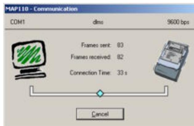
After completing the readout the meter data are displayed in the display area of the Landis+Gyr MAP110 Service Tool.
