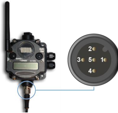
Figure 46: connecting the master receiver's 5-pin connector.
