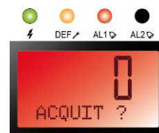
Figure 57: press ENTER on the reading to acknowledge an alarm.
