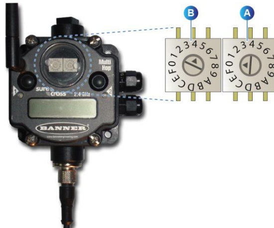
Figure 51: configuring the master receiver's address to @50.
