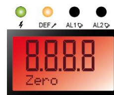
Figure 55: display in the event of a fault.
