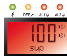
Figure 56: display after detecting high explosivity.
