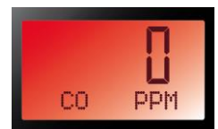
Figure 54: display under normal operating conditions.
