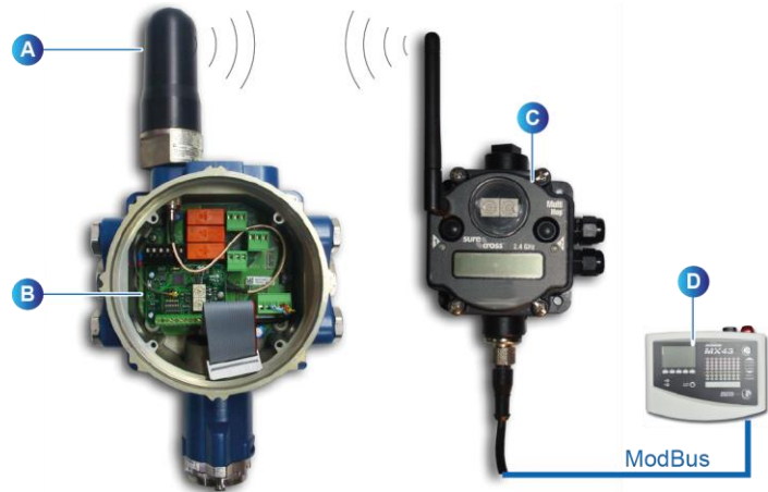
Figure 45: wireless OLCT 80 and master receiver (rep.C).
