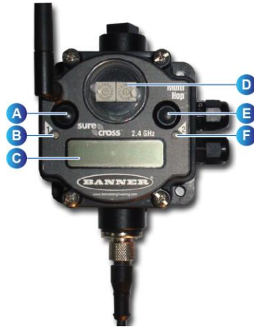
Figure 52: buttons and indicator lights on the master receiver.
