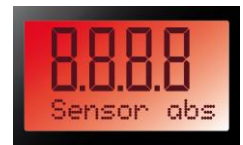
Figure 10: in the event of an alarm or fault, the type of fault is displayed. The orange DEF/ fault indicator light remains on as a solid light.
