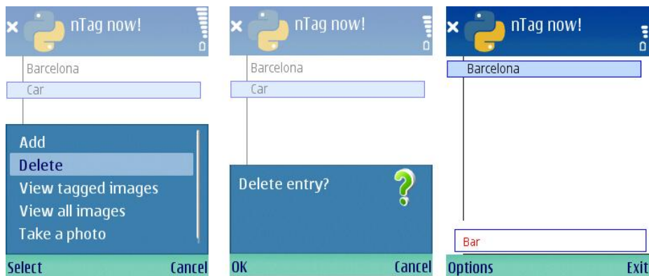
Figure E.5: Another case is to delete a tag. Here, these three screenshots demonstrate a whole procedure of deleting a tag – "Car". A query is promoted before the deleting operation is executed. After this, "Car" no longer exist in the tag list.
