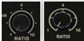
The Ratio parameter sets the amount of gain reduction. For example, if the ratio is set 2:1: this means for input level 2dB over the threshold, 1dB will be output.
