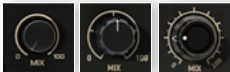
The Mix knob is a Dry/ Wet control. With Mix at 0%, you are hearing the uncompressed signal. At 100% you are hearing the compressed signal only. Intermediary positions will allow you to blend the level of compression.
