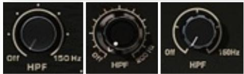
The High-Pass Filter (HPF) sets the frequency value at which to prevent prevent low frequencies triggering compression.
