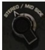
The FG-MU employs two processing methods for compression, Stereo & Mid/ Side.
