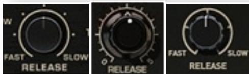
The Release parameter controls the offset point of compression - The speed at which the compressor stops compressing the signal, once it has fallen below the threshold value.
