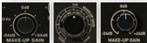
The Make-Up Gain parameter allows for adjusting the output level; to compensate for level reduction caused by compression.
