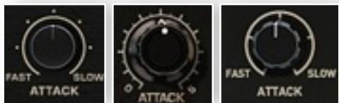
The Attack parameter controls the onset point of gain reduction - The speed at which compression occurs after the signal has exceeded the threshold value.
