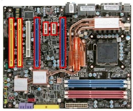
(The Highlighted slots are the PCIe slot available for RNX-N250PCe to install)
