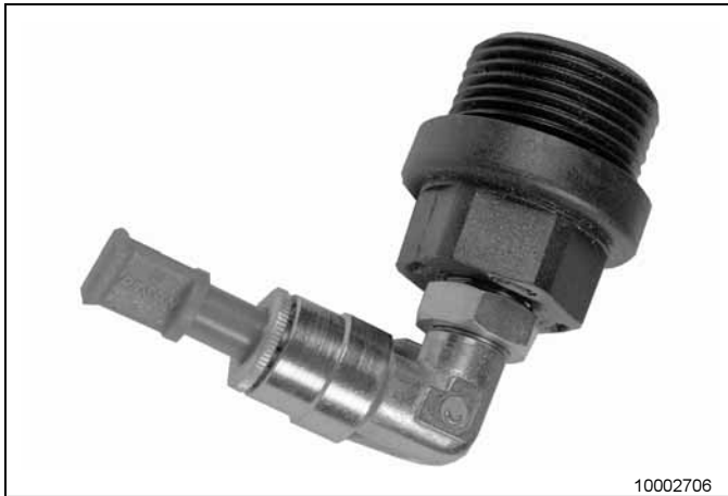
Fig. 102 Return-line connector, push-in type or screw type The return-line connection is designed to feed grease quantities that are not required back into the pump. It is installed instead of a closure plug (pump element).
