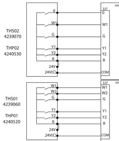
Trane THS01, THS02, THP01 and THP02 Thermostats are directly connected to RTRM board (J7 connector). TRANE THS02 and THP03 thermostats are directly connected to RTRM board (J6 connector).
