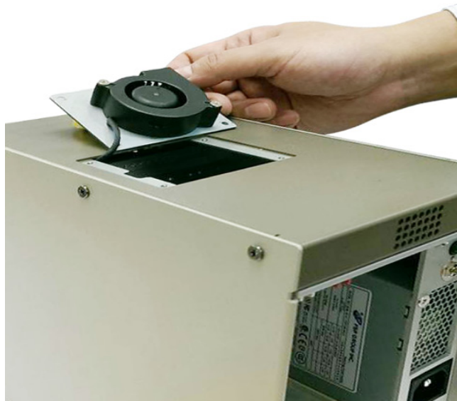
Figure 2.7 Top Cooling Fan
