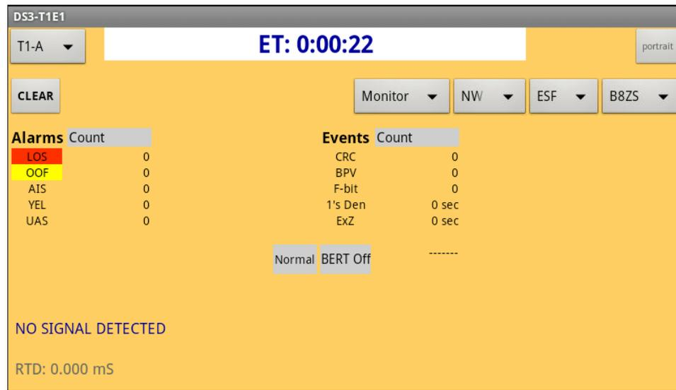
In the example above the unit is currently in Loss of Signal, the LOS is RED and No Signal detected is displayed at the bottom left.
