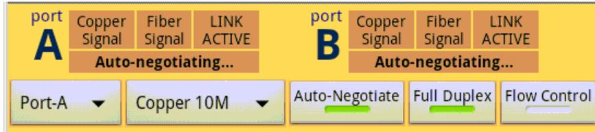
Along with LINK status the DataScout 10G highlights in bright white if there is Copper or Fiber signal detected and when there is a valid Fiber signal it displays the RX power in dB. Regardless of the selection of Copper or Fiber interface the Copper/Fiber signal will illuminate if signal is detected but the Copper/Fiber button indicates which port (Copper or Fiber) the DataScout 10G will RX and TX to/from.
