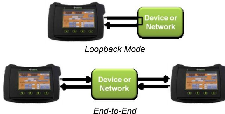
Select test mode by pressing the Menu key and select Looped (default) or End-to-End test
