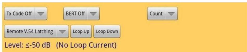
The test set will display the industry standard DDS/DataCom errors (AS,%AS, UAS, DGRM, Blk Size, BLK's, BLK Error and BLK rate) along with BERT pattern in Green if in Sync and Bit errors “0” next to the BERT pattern. A user can change the Bit count display by tapping on the **Count** pull-down menu and selecting one of the following:
