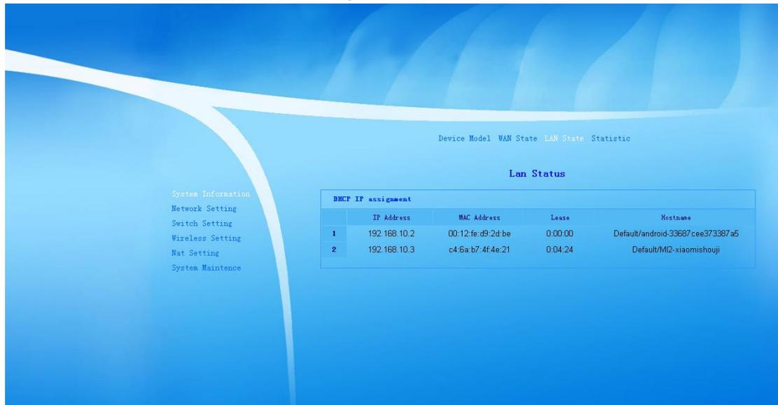
LAN Status shows current system LAN connection status, the situation that DHCP assigns IP address, connection to the system device hostname and so on.
