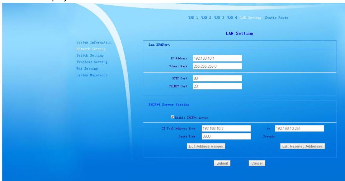
If you need make further subdivided management to IP Pool Address, to distinguish different devices assigned using address segment. You can click on edit address range, and enter DHCP IP address segment assignment setting section, it can assign IP address
