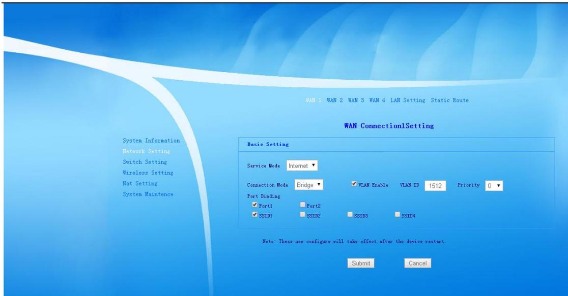
Router Mode: When connection type is router mode, you can obtain WAN side IP in three ways, to carry out related business. If using the most common PPPoE dial-up internet access, you can start VLAN enabling function and configure corresponding dial-up internet VLAN. Under routing setting, choose PPPoE in connection type, and input user name and password provided by ISP in PPPoE setting, then finish PPPoE setting. As displayed below.
