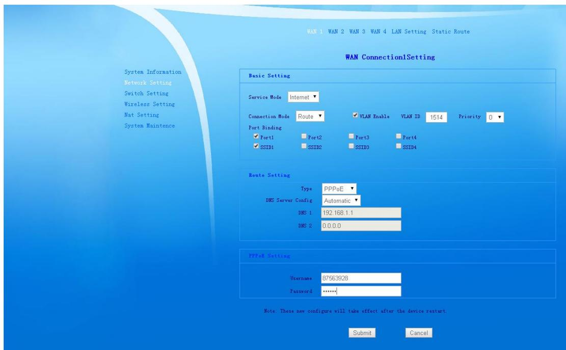
Router and Bridge Mixed Mode: As the following figure configured, WAN 1 is set to Bridge Mode, IPTV terminal connected Port 1 and SSID 1 carry out multi-broadcast stream media communication. WAN 2 is set to Router Mode, required internet terminal connected Port 2 and SSID 2 is for internet business. Please refer to Bridge Mode and Router Mode setting for detailed configuration.
