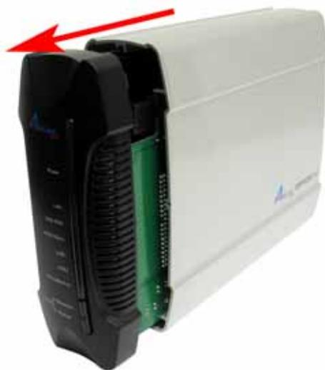
**Step 3** Put the 3.5-inch IDE or SATA hard disk into the slot, and connect the proper data cable for your hard drive. (The red cable is used for SATA and the gray one is for IDE).
