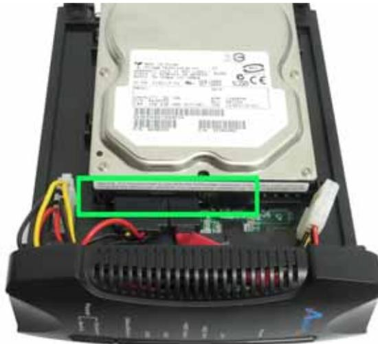
**Step 4** Secure the drive to the metal plate on the sides with the provided four screws.
