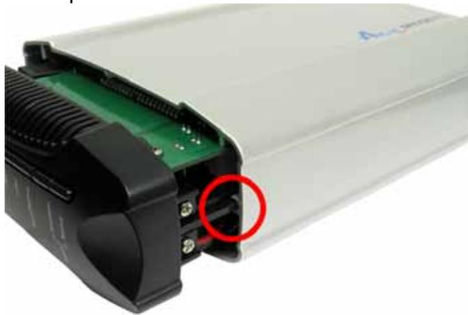
**Step 6** Re-attach the back panel to the device and secure it with the two screws removed in step 1.
