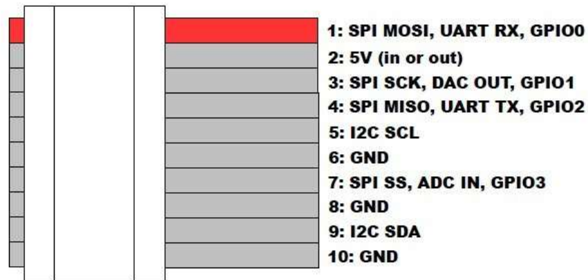
Figure 10 – Pixy's pin layout for the I/O ports [10] (Permission Obtained from Charmed Labs)
