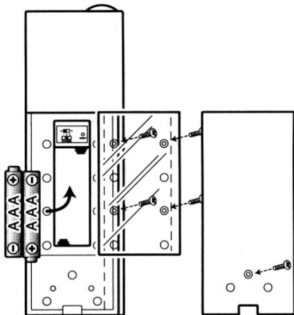
1. Remove the screws on the battery compartment.
