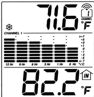
If no signals are received, blanks are displayed. Press **CHANNEL** and **MEMORY** simultaneously to enforce another search. This is useful in synchronizing the transmission and reception of the remote and main units.
