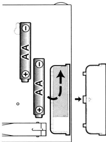
3. Replace the battery compartment door.
