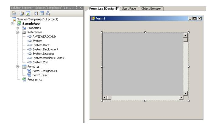
The Interop.VIEWEROCXLib.dll is automatically generated when launching an MS Studio project that uses the PDFViewer Class and ViewerOCX.dll is registered on that OS.
