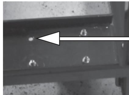
Remove rear inside nut and bolt from both swivels casters.
