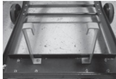
Using original nuts and bolts, install drip pan brackets.
