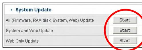
For system update, users must have new firmware in PC. Access FW-1120 by web browser on user PC, go to admin > utility > system update menu and click "start" button to start firmware update. After completion of update, FW-1120 must be rebooted for updated firmware to apply.
