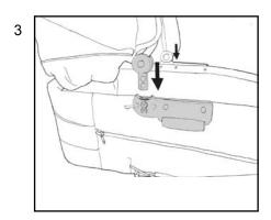
Attach the hood to the pram body by pushing the plastic leg of the hood into the plastic holders on the pram body. Make sure they snap into place.
