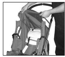
• Place the seat unit fabrics over the chassis, using the zippers and press-studs, located on the fabrics.
