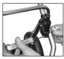
• Remove the screws that hold the front bar and save them for future use. They will be needed again when the seat unit is reassembled.
