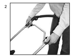
Release the chassis locks, located on both side of the handle, by pulling the black plastic parts up towards you with both hands.
