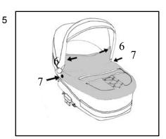
• Press the apron onto the hood (6) and onto the plastic holder (7) on each side.
