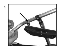
• Fasten the other end of the adapter with the screw and domed cap which comes with the adapter. Do not tighten the cap too tight, but leave 0,5 mm, so that the chassis can be folded.
