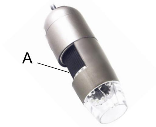
When the object is located at the top of the front cap, there are two focus positions, each with different magnification power, can be found by rotating the focus knob.
