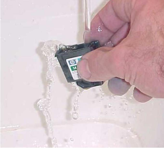
There is a small sponge in the bottom of the printhead. In order to completely clean it, the tank should be rinsed thoroughly after soaking. Run warm water in the open top of the tank. **MUCH INK** will run out during rinsing. It may take several minutes to clear.
