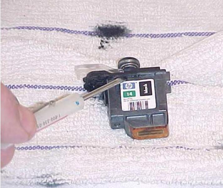
Once the top of the printhead is loose, gently pry the top piece apart from the tank.
