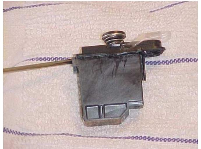
Place the screwdriver in front where the round piece was and pry to make the final separation
