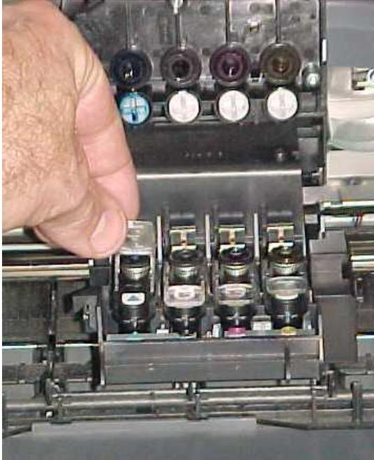
Lift the tab on the front of the printhead to remove.
