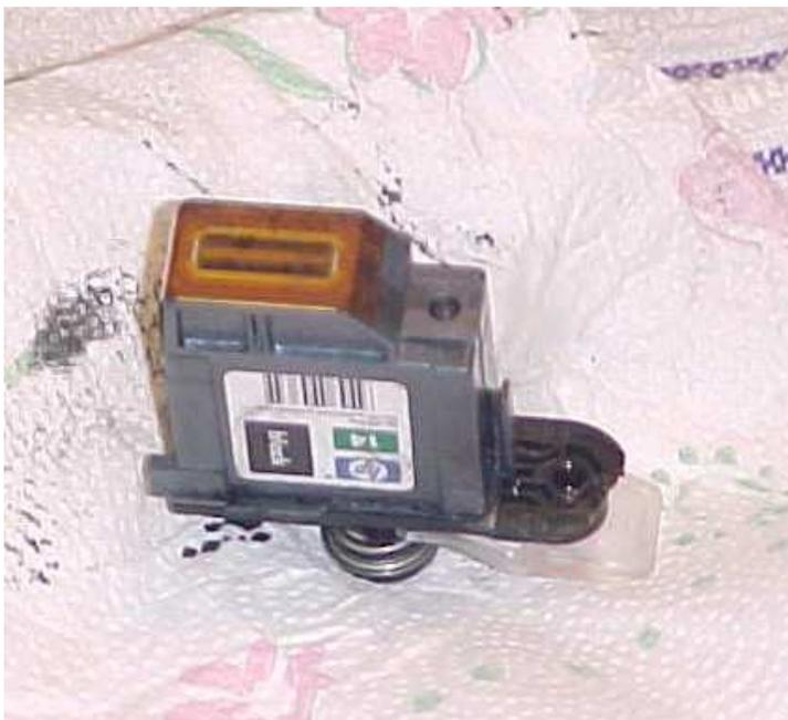
Thoroughly clean off the printhead including the contacts, and the bottom where the ink comes out. Replace the round piece, it should snap into place. Let the printhead set for several minutes. The ink should stop flowing out of the bottom. Clean and replace the printhead in the printer and test. It may take several pages to clear and function properly.
