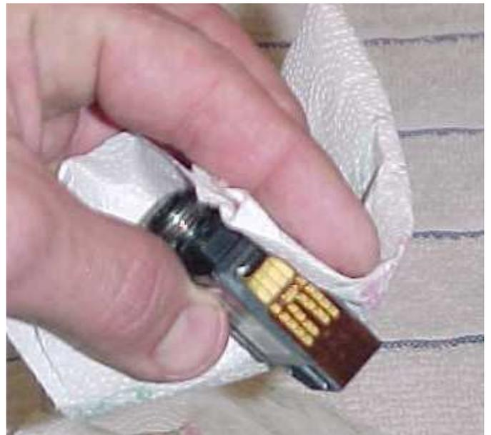
Smear the bottom the printhead across paper towels to clean access from the ink dispenser. Some dripping may occur. Repeat until dripping stops and contacts are clean and dry. Let stand a few minutes then replace printhead in printer and test.
