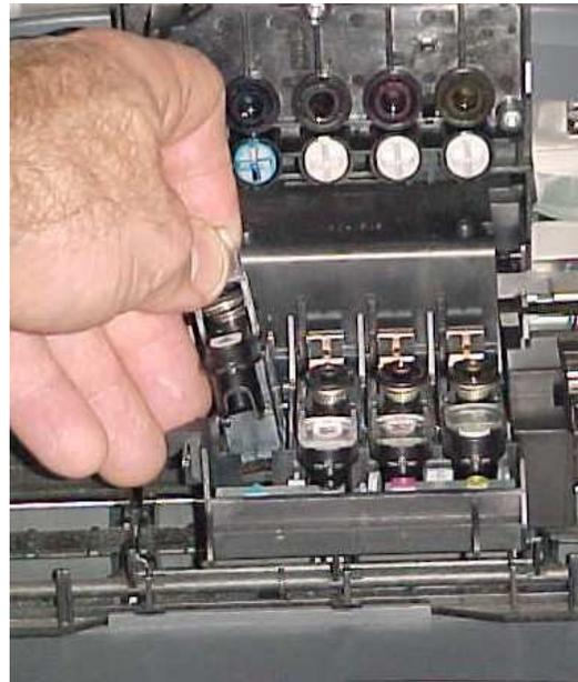
Gently remove the printhead from the carriage for service.
