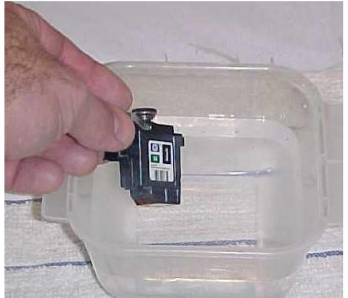
Soak entire printhead in water for several minutes. Small amounts of ink will seep out of the printhead.
