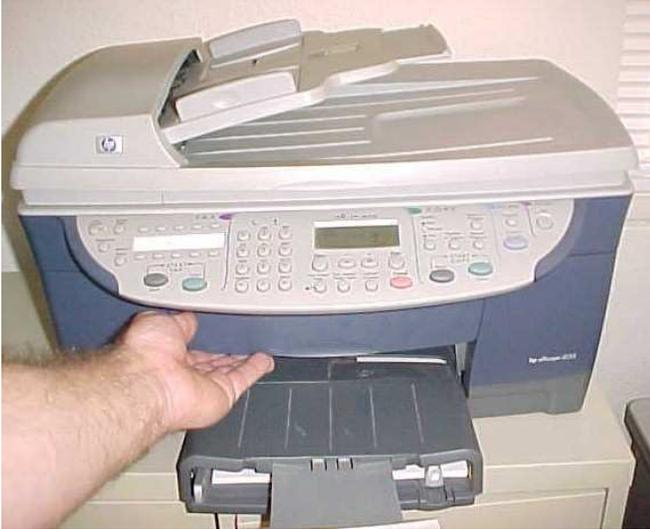
To access the ink system you must open the front cover of the unit. There are no latches to release. Simply lift up on the door located above the paper tray.
