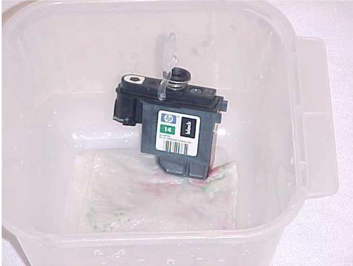
Place a paper towel in the bottom of a bowl and cover the bottom with warm water. Place the bottom of the printhead in the water for several minutes. Dry completely and test the printhead .
