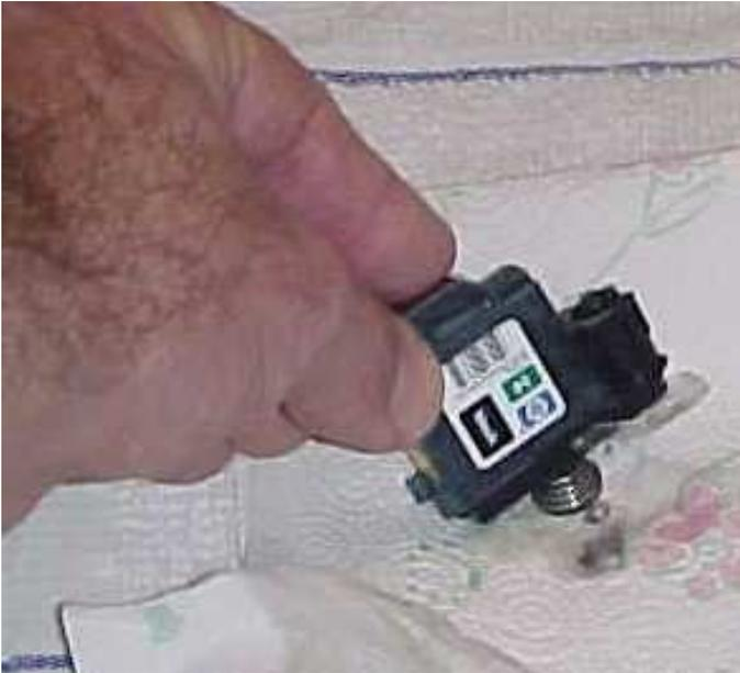
Lightly tap the top of the printhead on a small pad of paper towels. HP !4's have a spring release at the top for ink flow.
