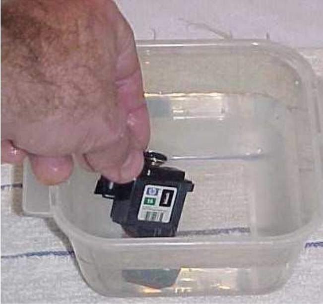
Remove the printhead from the water after several minutes.
