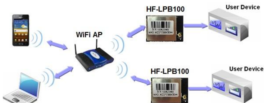
Figure 9. HF-LPB100 Basic Wireless Network Structure
