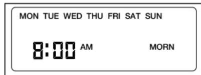
3. Press either v or ^ button to adjust the time setting for MORN. (Note: Holding down either v or ^ button scrolls the time in 30 minute increments.)
