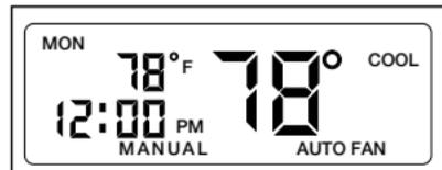
2. Press QUICKSET button. The display will show all the days of the week at the top of the display. This signals that you are in QuickSet™ mode. "MORN" is the first setting for the day. The display will show the setpoint time.
