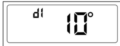
6. Press either  $\nabla$  or  $\blacktriangle$  button to change the first stage temperature differential. The differential may be adjusted from .5°F (05°), 1°F (10°), 1.5°F (15°), or 2°F (20°). (If your system cycles too often, increase the temperature differential setting.)
