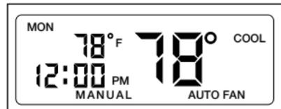
3. To advance through each day's programmed setpoint times, temperatures, and fan settings continue to press the SET button. Each time you press the SET button, the LCD display will advance to the next setting in the program.
