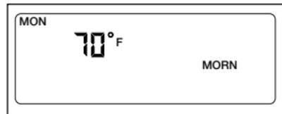
6. Press either  $\nabla$  or  $\blacktriangle$  button to adjust the temperature setpoint for the programmed MORN time.
