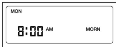
4. Press either  $\nabla$  or  $\blacktriangle$  button to adjust the time setting for MORN. (Note: Either  $\nabla$  or  $\blacktriangle$  button scrolls the time in 30 minute increments.)
