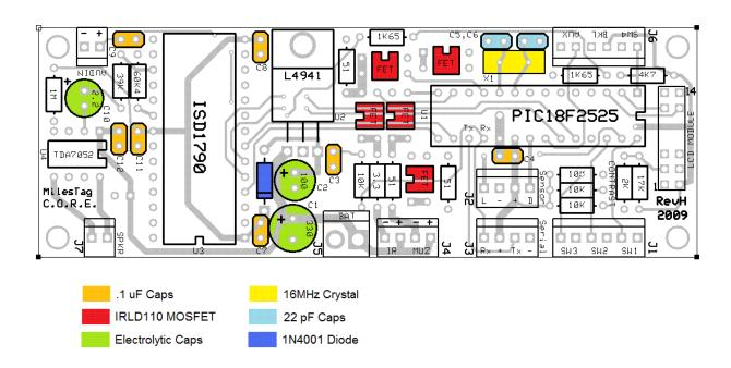
**Note 1**: Use a mica insulator between the L4941 regulator and the PCB. **Note 2**: The 1N4001 diode is only on the newer manufacture PC boards.
