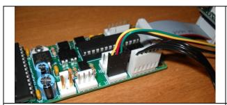
Attach adapter cable to the RevH Main Board. The pinout matches the extension cable sold by acroname. *NOTE: For RevG boards the serial connector pinout is different.*
