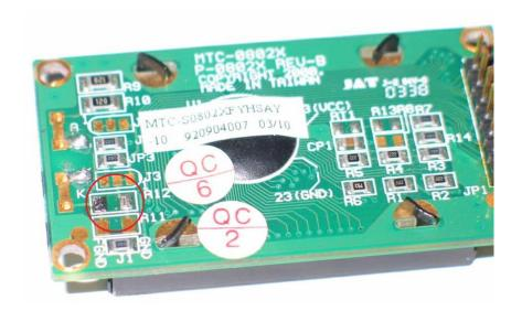
Other LCD modules may require installation of a current limit resistor (this is the case with some units from Crystal Fontz). Refer to the manufacturer datasheet for information.
