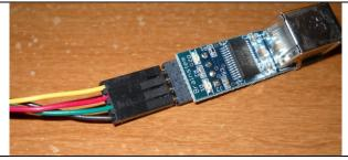
Here is the connection to the Acroname USB interface. The adapter is powered by USB. If you are using a RevH board as your Referee controller, you can install the USB adapter in the same case.
