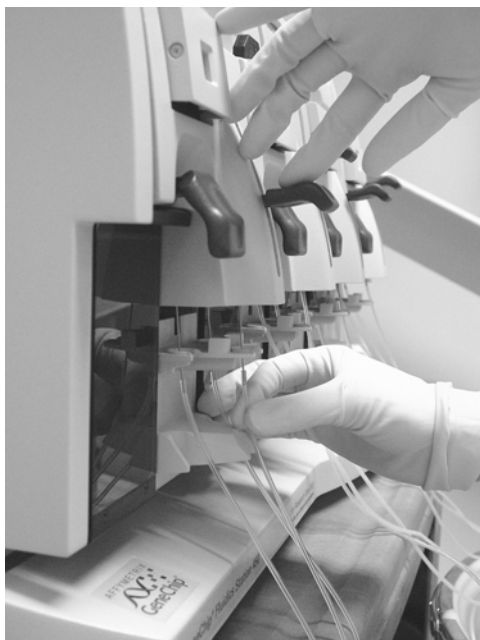
Figure 4.1.2 Inserting tubes on the needles. Take care not to break or bend the needles.
