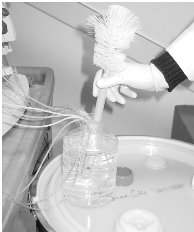
Figure 4.1.4 Tamp down on the tubes to ensure that the ends remain immersed in the solution.
