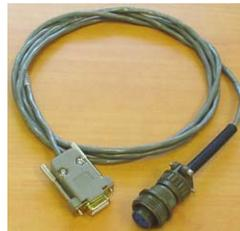
NMEA Input Interface test cable
