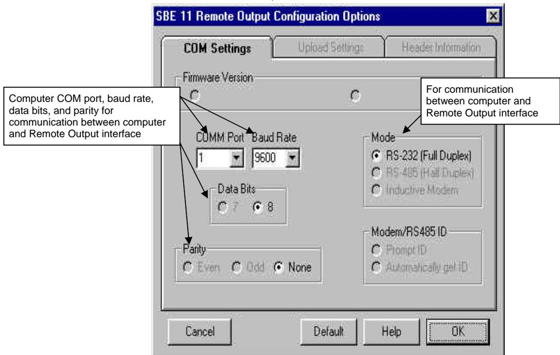
Make the selections in the Configuration Options dialog box to correspond to the information on the Deck Unit Configuration Sheet. Click OK to save the settings.
