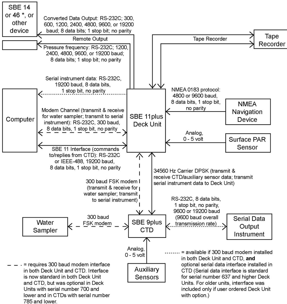
Note: A NMEA navigation device can be connected directly to the computer instead of to the Deck Unit. This feature is supported in Seasave V7 version 7.17 and later. The output from Seasave is the same, regardless of whether the NMEA data was appended in the Deck Unit or in the computer.
