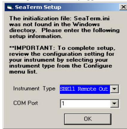
Select the instrument type (for example, SBE 11 Remote Out if connected to the *Remote Out* connector) and the computer COM port for communication with the instrument. Click OK.
