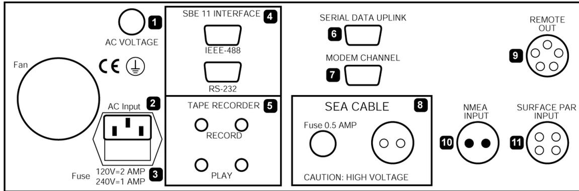
**1 AC Voltage Switch Selector** - select 120 VAC or 240 VAC 50/60 Hz
