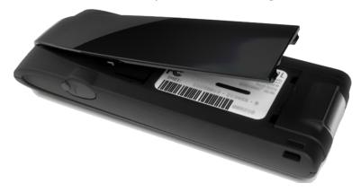
2 Insert the 4G SIM Card with the contact points (typically gold-colored) facing toward the device. Position the card with the notched corner as circled below and slide the card into the slot.
