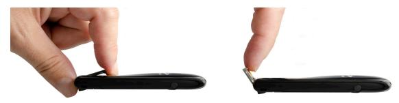
4 Hold the device along the side edges and gently insert the device into your computer's USB port. The MC551 modem should fit easily into the port. Do not force the device into the port as this might damage both the device and the port.
