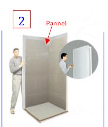
Move the Pannel (2) to fit it over the Base's rubber. Check its alignment and place the corresponding screws. not tight.
