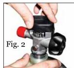
Tighten valve by hand. Make sure the metal of the tank touches the metal of the valve. (Fig. 3)
