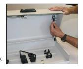
on the door. For vertical installations, you should remove the bottom spring on a RAD 4 to avoid interference with rifle stocks. You may also opt to remove the top gas springs in vertical installations. If you ever need to remove a gas spring, pull up on the small black spring clip with a small screwdriver or needle nose.
