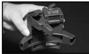
In these electronic meters, the optical port is too close to the dome's outer rim for it to be possible to position the Sensor Head over the port, because the Sensor Arm is too long, even when fully pushed in.
