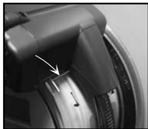
13. Tighten the hose clamp so that the Sensor Unit is snug but can still move easily.
