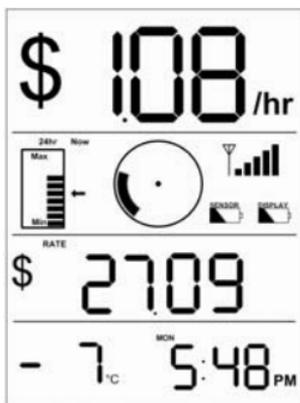
Pressing the MODE button on the back of the Display Unit toggles the display between Kilowatt mode and Dollars & Cents mode.
