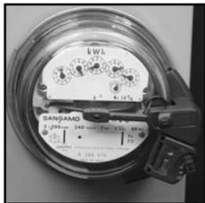
*NOTE: If the Sensor Arm is not properly positioned, the Sensor Unit may not detect the motion of the disk and will generate incorrect readings.*
