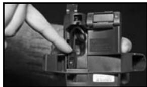
6. Tuck the wire neatly into the side cavity.
