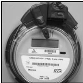
If the Sensor Unit indicator does not begin to flash irregularly after about 5 minutes, the Sensor Arm is not properly positioned over the optical port or the glass dome is dirty. Repeat steps 10 and 11 above.
