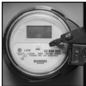
6. Tighten the strap adjustment screw until the Sensor Unit cannot be moved easily. Do not over-tighten!
