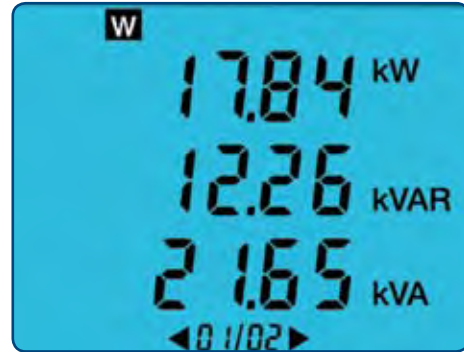
Displays all power measurements on one screen.
