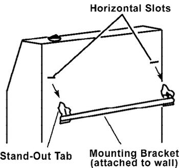
**Figure 11 - Mounting Heater Onto Mounting Bracket**
