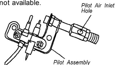
**Figure 24 - Pilot Inlet Air Hole**
