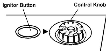
Figure 16 - Control Knob in The OFF Position
