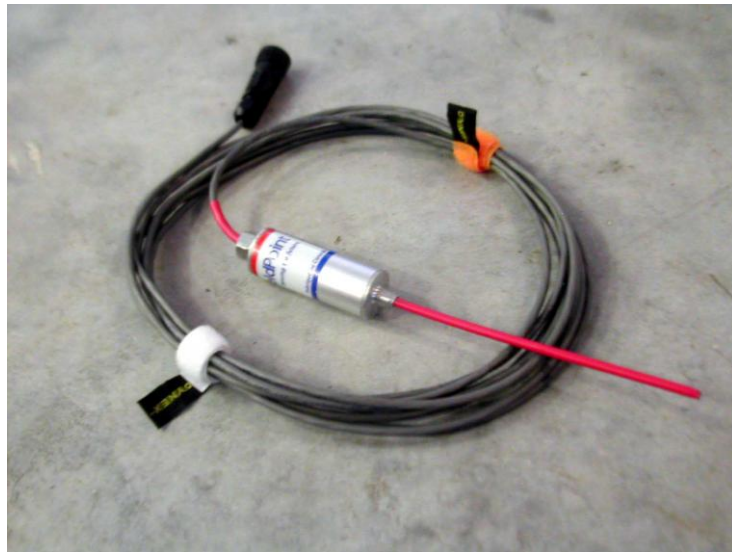
Figure 1. The magnetostrictive displacement sensor. The extended red probe is the waveguide.
