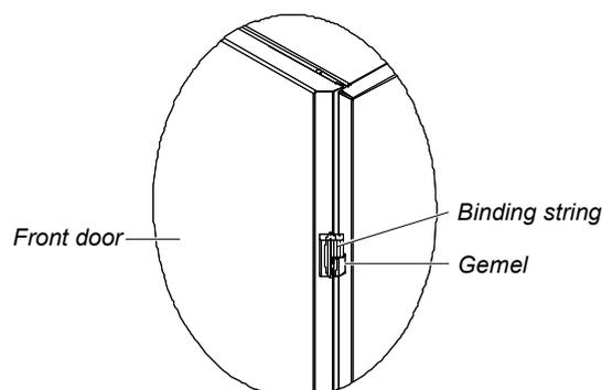
Figure 2-27 Binding string of front door
