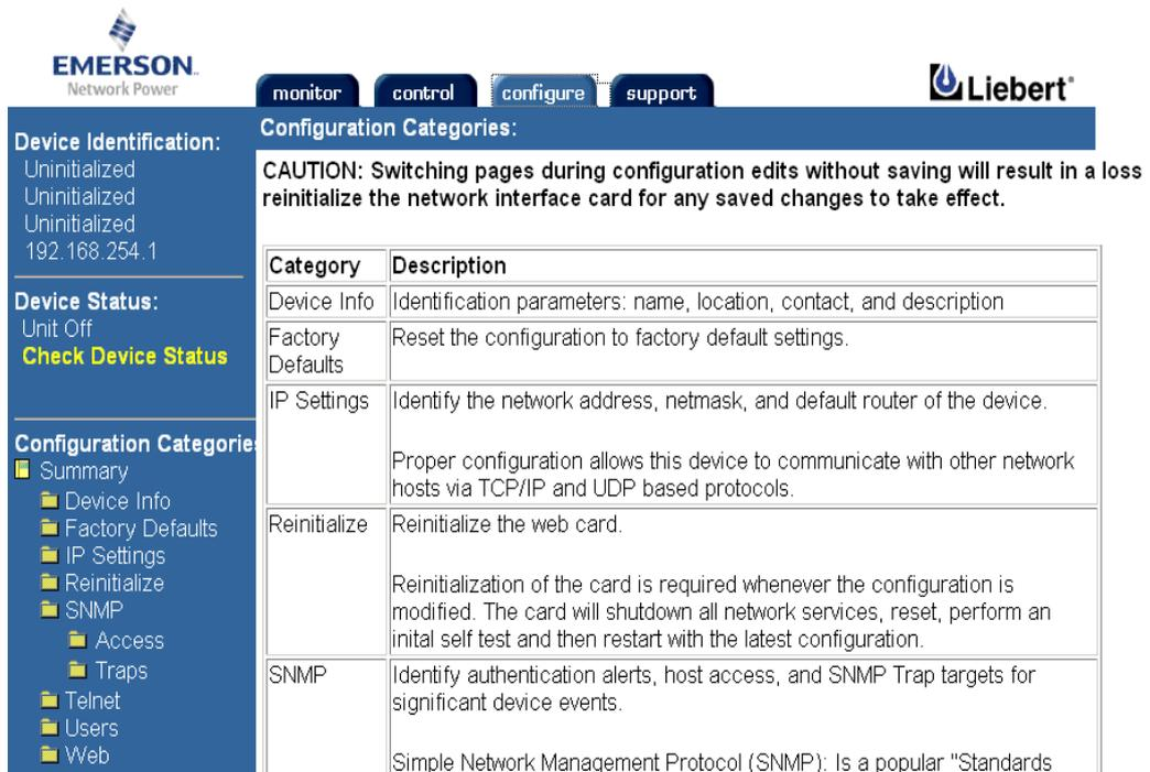
Figure 6-10 Configuration interface
