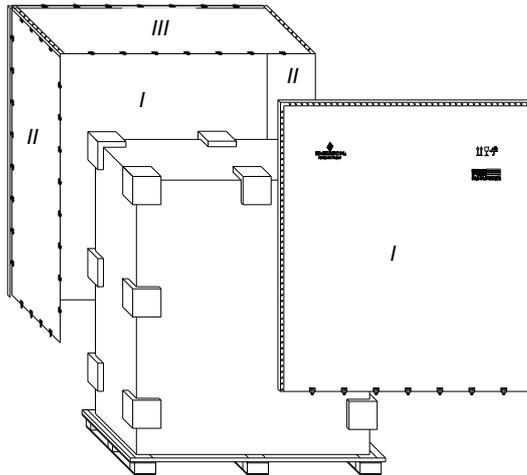
Figure 2-4 Removing side boards and top cover
