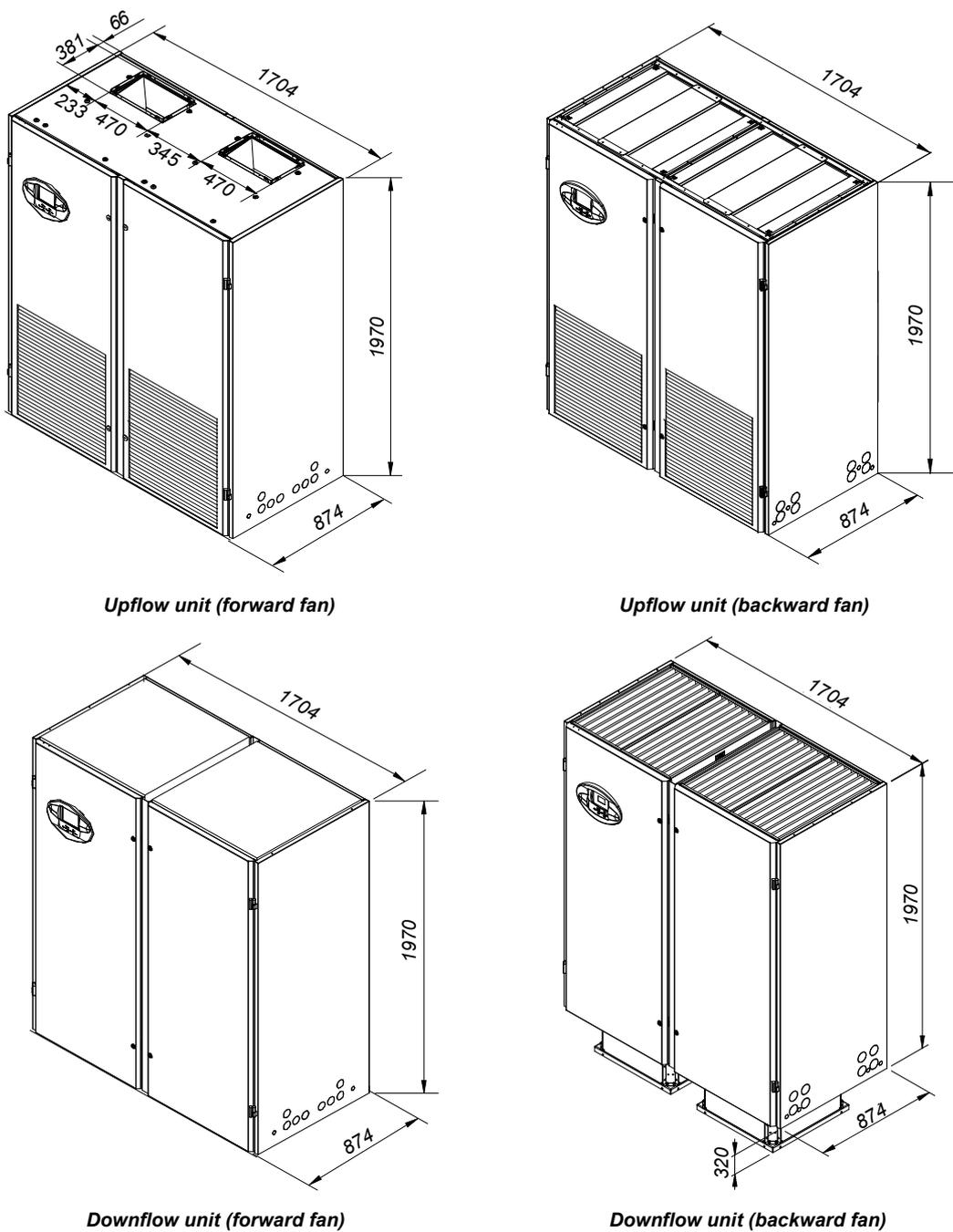
Figure 2-8 Two-bay series (unit: mm)
