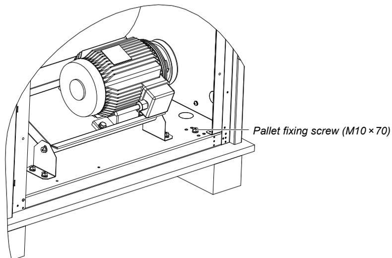
Figure 2-5 Fixing screw position of pallet
