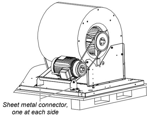
**Figure 2-29** Transportation fan unit binding screw
