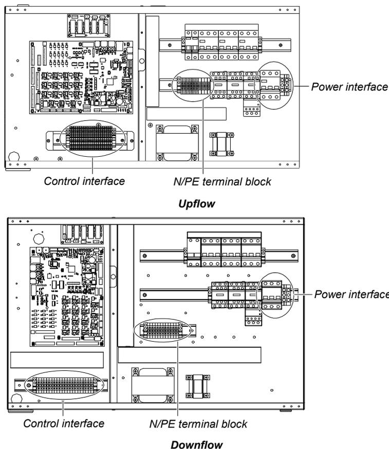
Figure 3-1 Electrical control box interfaces of one-bay series
