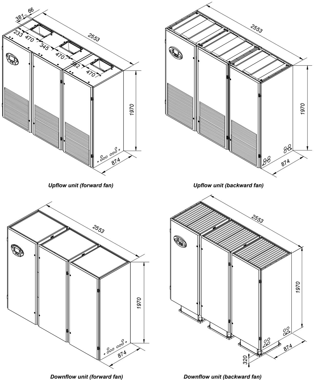
Figure 2-9 Three-bay series (unit: mm)
