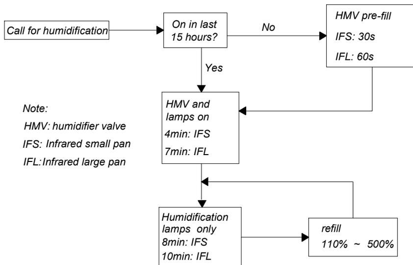
Figure 7-4 Humidification control logic
