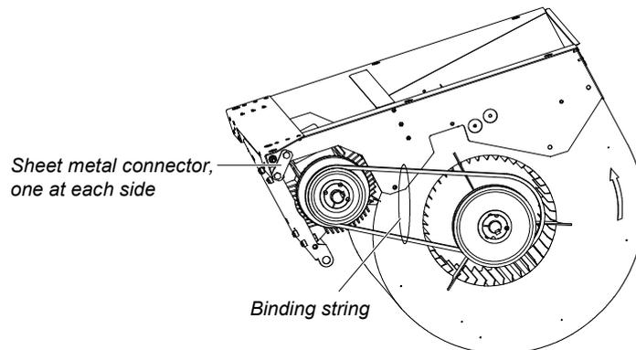
**Figure 2-28** Transportation fan unit binding screw and string
