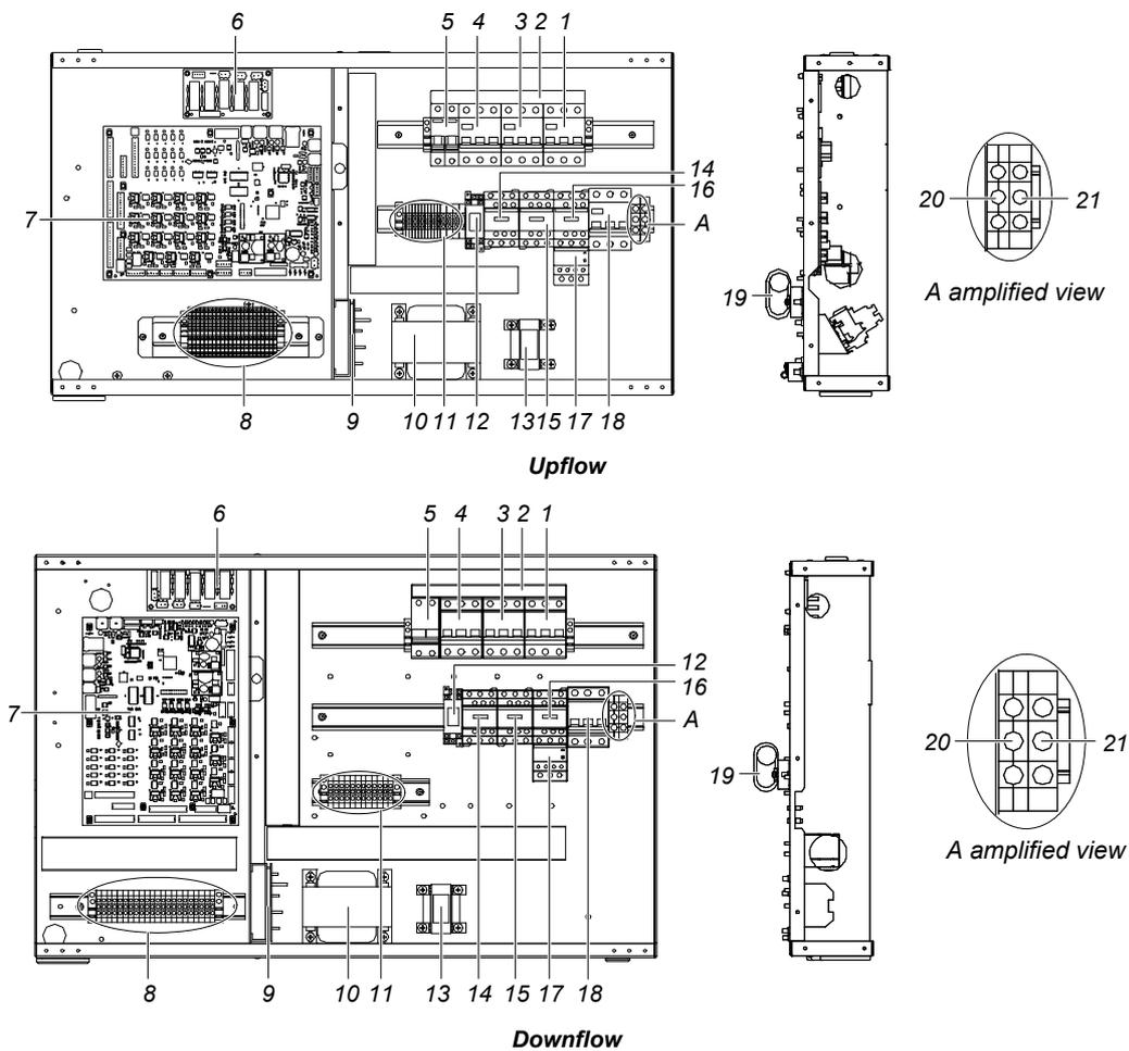
Figure 1 Internal structure of one-bay series electrical control box
