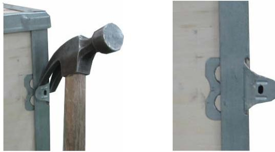
Figure 2-3 Straightening the hook
