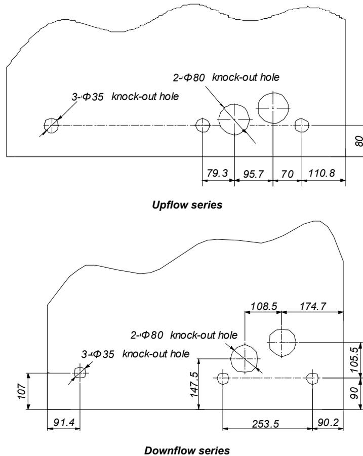
Figure 2-16 Knock-out holes of side panel (unit: mm)
