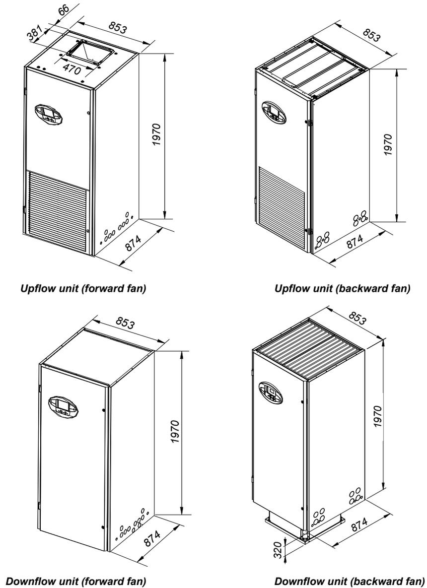
Figure 2-7 One-bay series (unit: mm)
