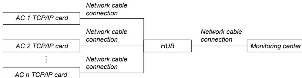
Figure 6-14 Networking figure of TCP/IP communication card
