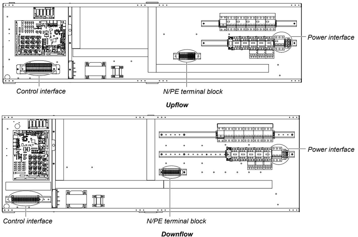
Figure 3-3 Electrical control box interfaces of three-bay series
