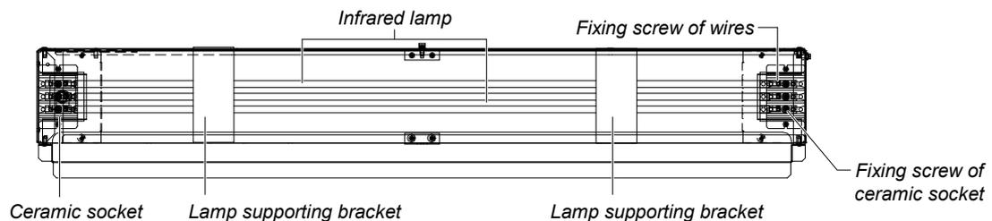
Figure 7-3 Lamps of infrared humidifier
