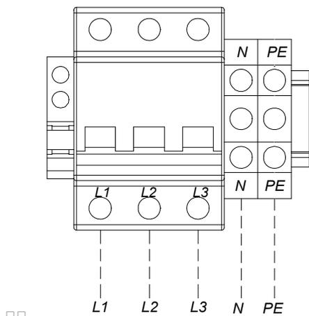
Figure 3-4 Amplified figure of power interface
