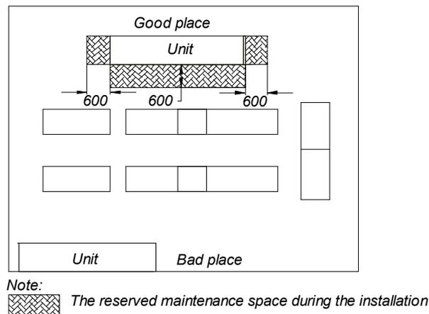
Figure 2-17 Installation place of indoor unit (unit: mm)
