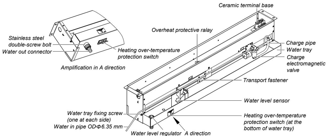
Figure 2-25 Infrared humidifier
