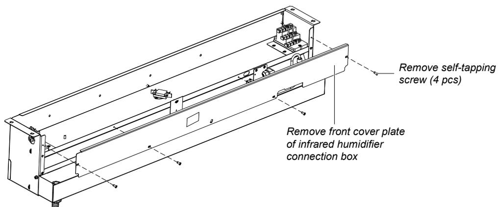
Figure 2-32 Opening front cover plate of the connection box
