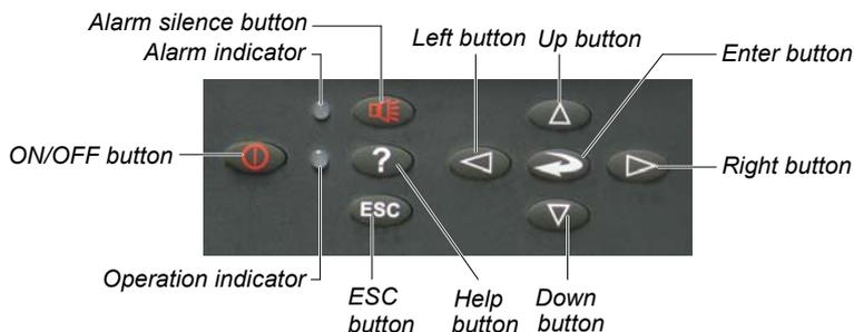
Figure 5-1 Button and indicator panel
