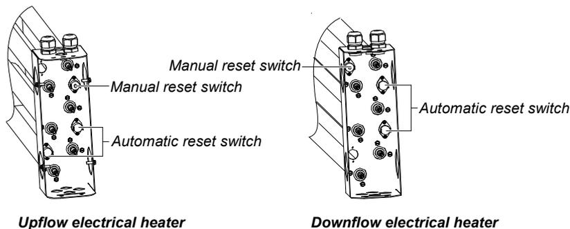
Figure 7-5 Upflow and downflow electrical heater
