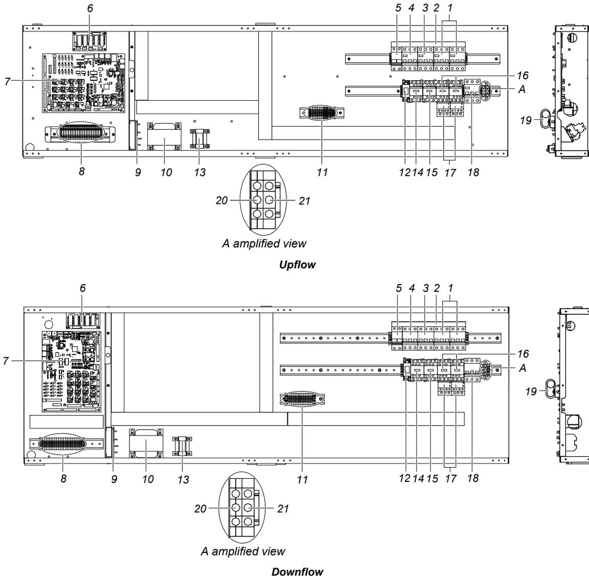
Figure 2 Internal structure of two-bay series electrical control box
