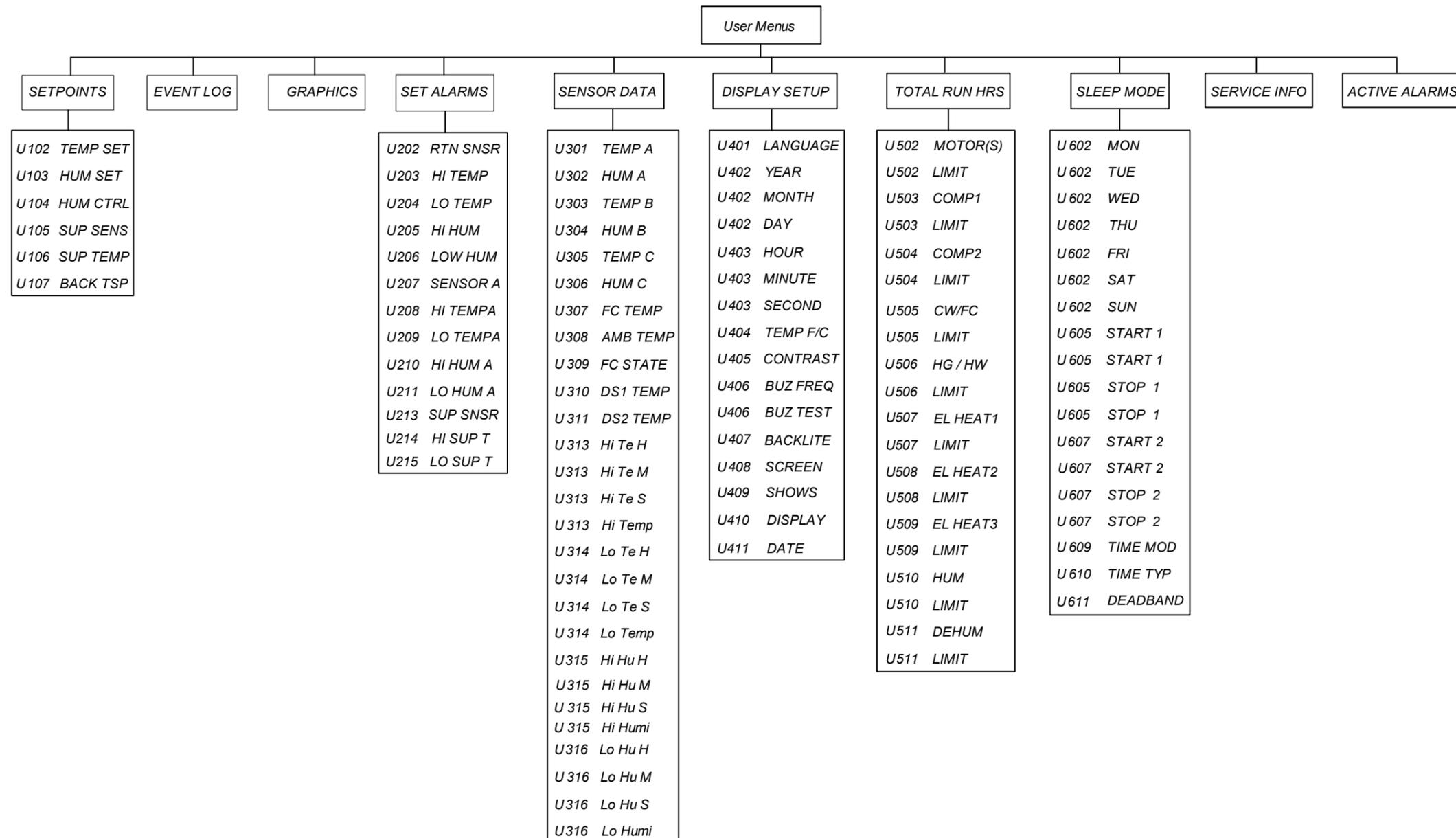
Figure 5 Structure diagram of user menu
