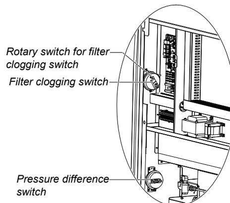
Figure 7-2 Filter clogging switch and pressure difference switch
