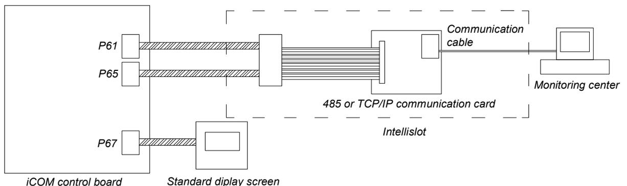
Figure 6-4 Electrical schematic figure of host communication configuration
