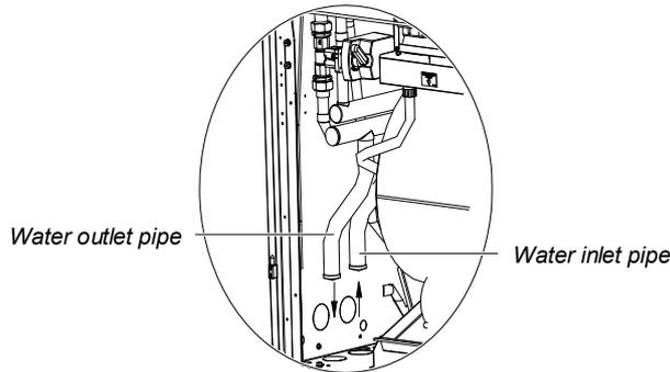
Figure 2-26 Welding figure of chilled water in and out pipes
