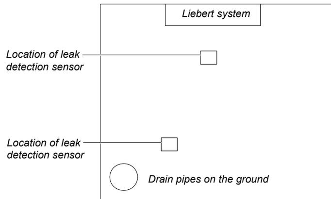
Figure 7-1 Recommended location for the water leak detector
