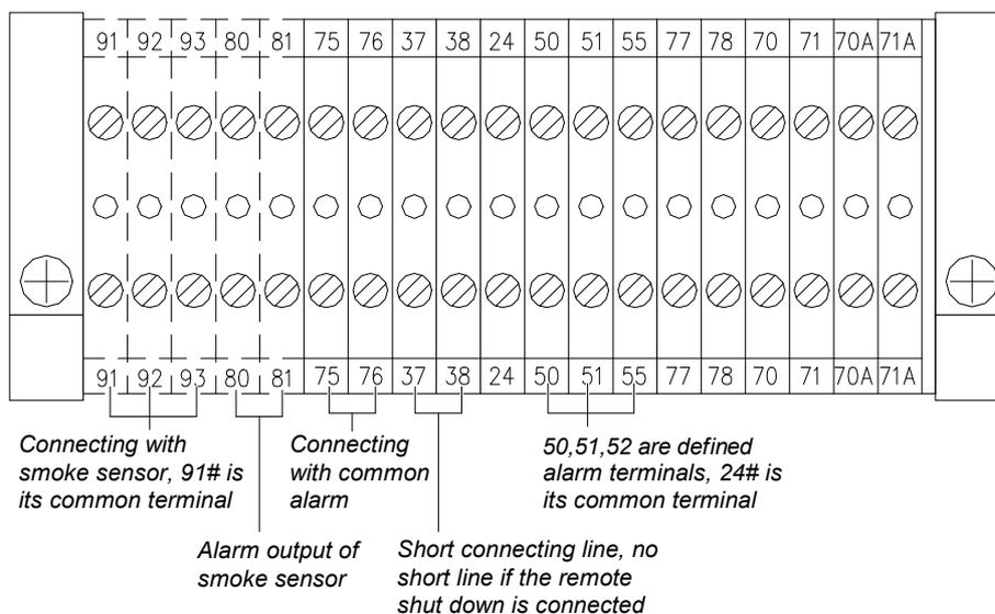
Figure 3-6 Wiring of control interfaces
