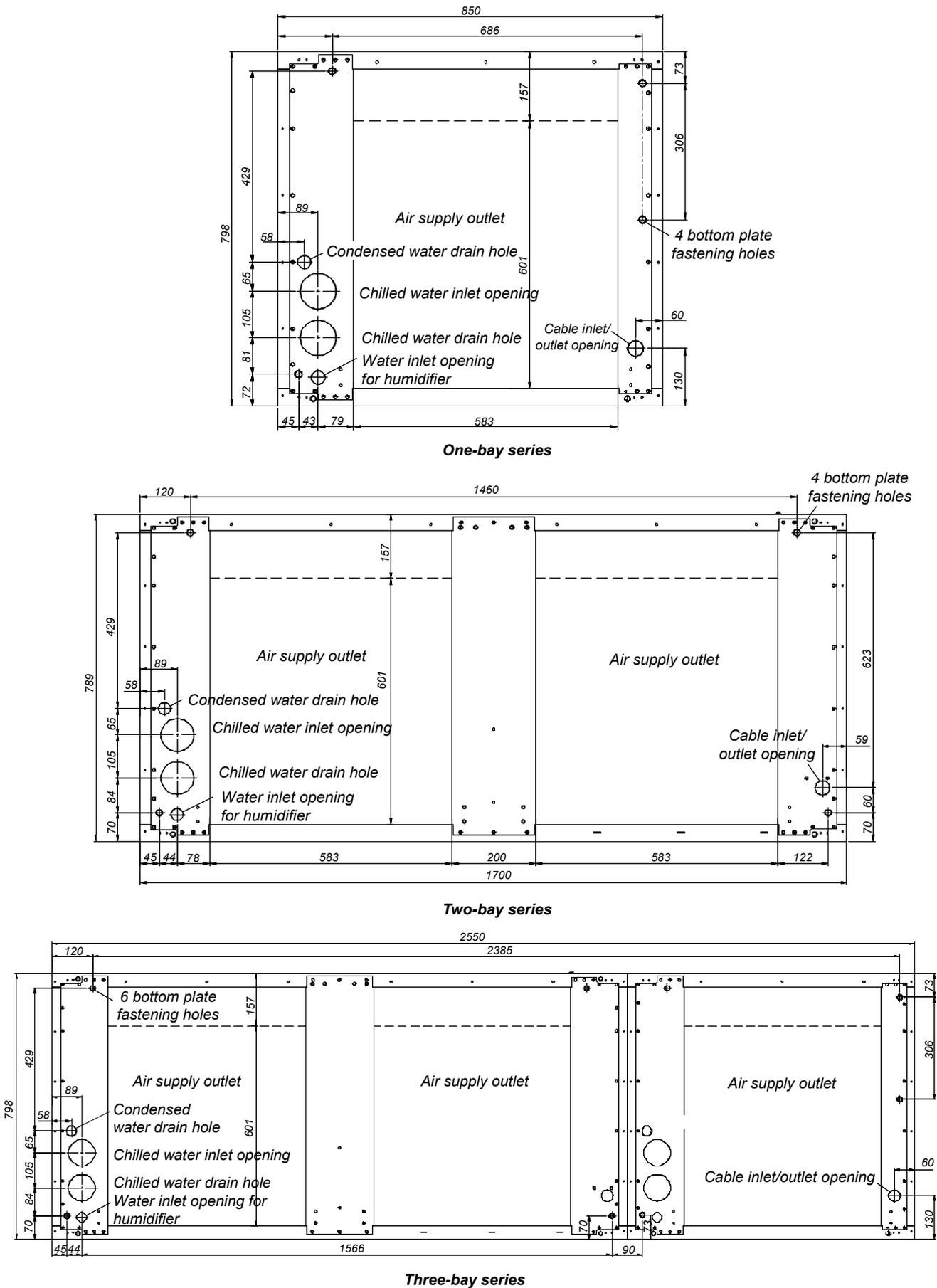
Figure 2-15 Base cut-out locations of the backward fan downflow series (unit: mm)
