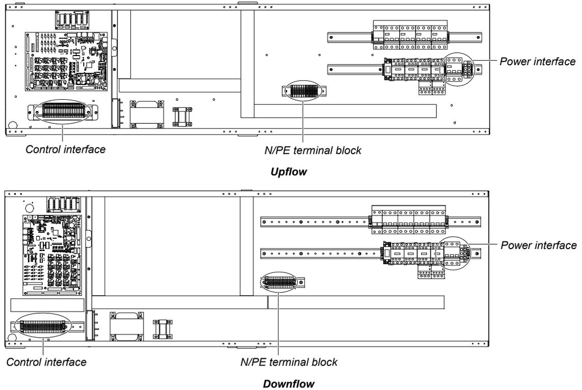
Figure 3-2 Electrical control box interfaces of two-bay series
