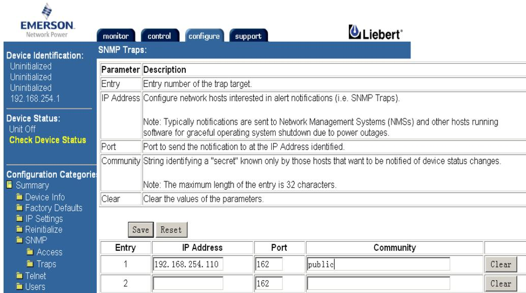
Figure 6-13 NMS configuration interface of SNMP host monitoring center (2)
