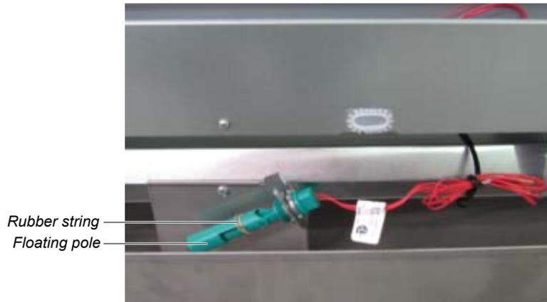
**Figure 2-34** Floating pole of the high water-level sense switch
