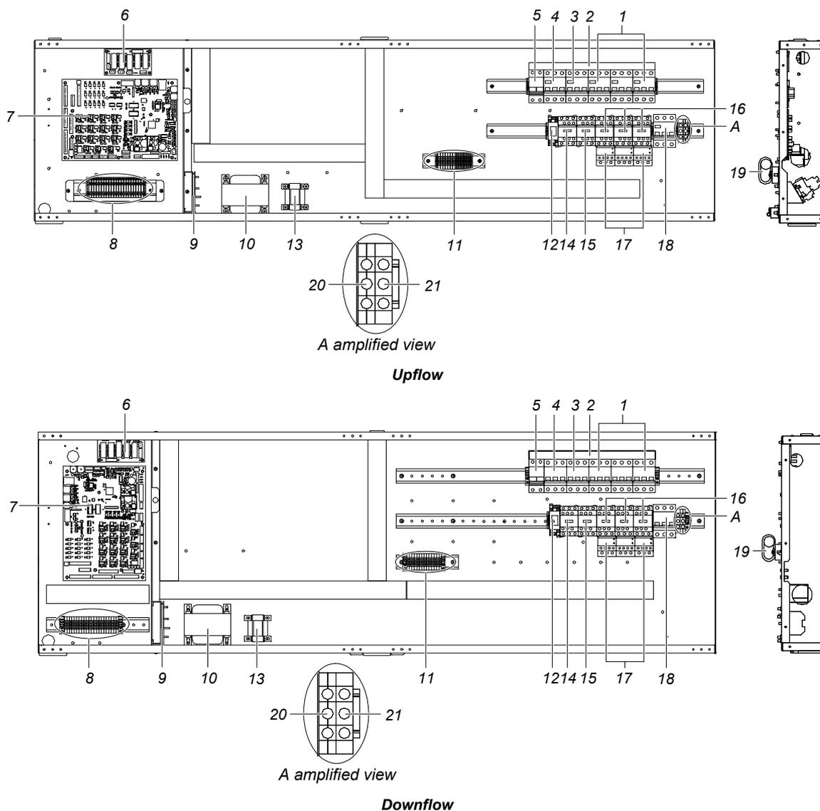
Figure 3 Internal structure of three-bay series electrical control box
