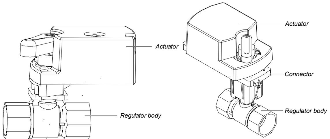
Figure 7-6 Water flow control valve
