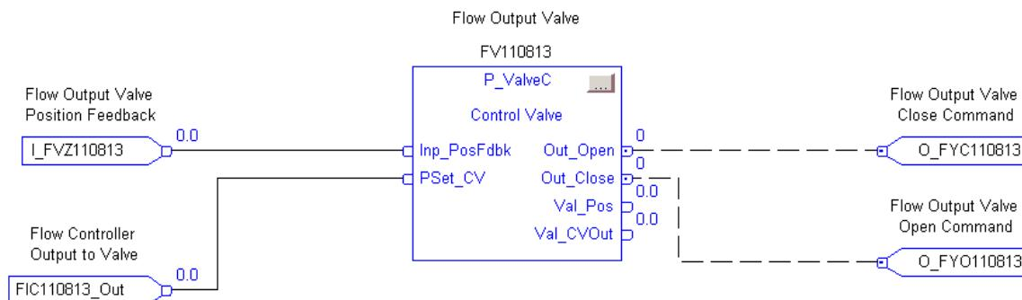
In this example, the field inputs for position feedback are wired (or connected) to the instruction input Inp\_PosFdbk. Out\_Open and Out\_Close are connected to the field outputs going to the valve. The input to the instruction to set valve position is wired to PSet.CV. Cfg\_ProgDefault is set to 1 so the instruction defaults to Program mode.
