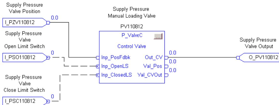
The field inputs for position feedback, open limit switch, and closed limit switch (as shown in the illustration) are connected to the instruction inputs Inp\_PosFdbk, Inp\_OpenLS, and Inp\_ClosedLS. The Out\_CV is connected to the field output going to the valve.
