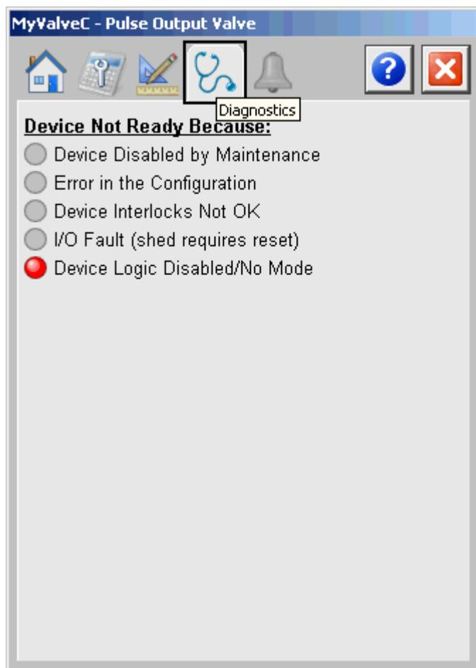
The figure above shows that the valve is not ready because the Device Logic is disabled or there is no mode.
