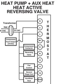
NOTE: When switched to HP mode, W1 is connected internally to Y1.
