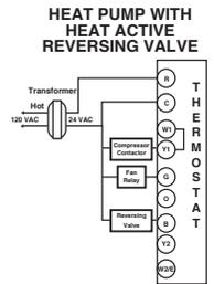
NOTE: When switched to HP mode, W1 is connected internally to Y1.
