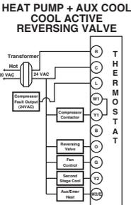
NOTE: When switched to HP mode, W1 is connected internally to Y1.
