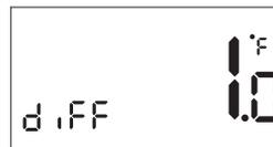
6. Press SET. The display will switch to the differential setting for 2<sup>nd</sup> stage heating and cooling.
