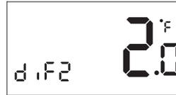
8. Press SET. The display will switch to the differential delay.
