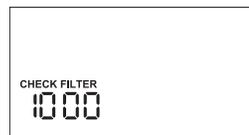
14. Use the ▲ or ▼ to adjust the filter timer from 0 (OFF) to 9900 hours. **NOTE:** The filter timer is based on equipment run time. Select the length of time based on the recommended service interval for your filter.
