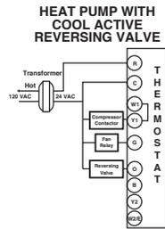
NOTE: When switched to HP mode, W1 is connected internally to Y1.
