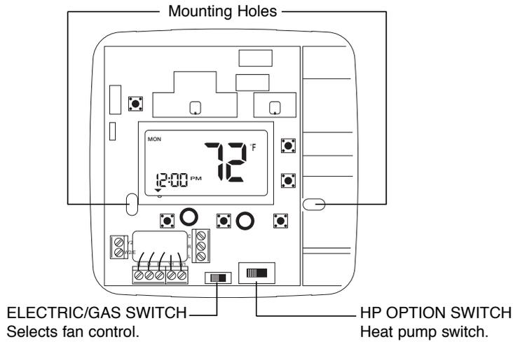
6. Mark placement of mounting holes (see Figure 3). Set base aside.
