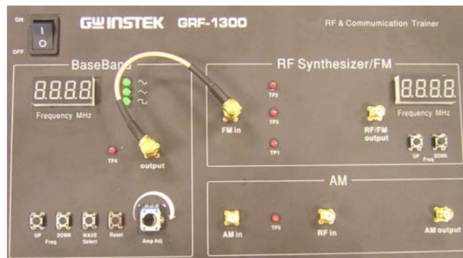
Figure A-3. Connection diagram between different modules
