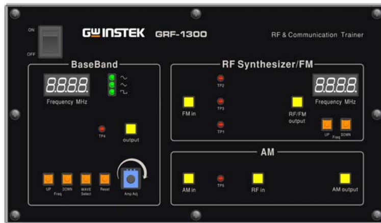
Figure A-1. The GRF-1300 control panel
