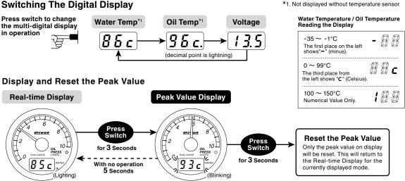
\*Peak readings are reset when the key is turned OFF.
