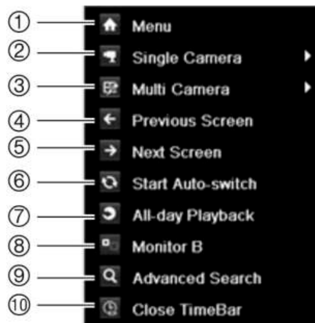
Figure 11: The mouse menu for the main monitor
