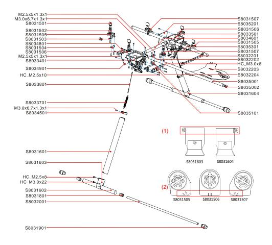
Note: (1) Left and right T-Frame are different; (2) Left set, middle set and right set of carbon tube bracket are
