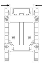
2. Lift loudspeaker up and off.
