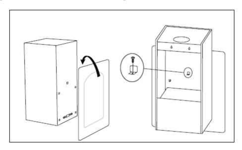
**2)** Position the hood against the wall that you are intending to install it on and mark the position of the screw holes that are to be drilled.
