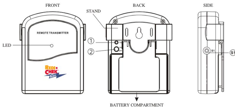
STAND – Swings out and allows you to stand transmitter on tabletop.
