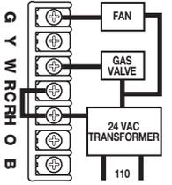
**TYPICAL COOLING AND HEATING SYSTEM (4-WIRE)**
