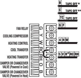
\* If replacing a Honeywell TM-11, tape off wire "R"; connect wire "B" to terminal "RH".
