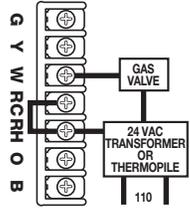
**TYPICAL HOOKUP FOR 3-WIRE HEAT SYSTEM IF THIRD WIRE IS FAN WIRE**
