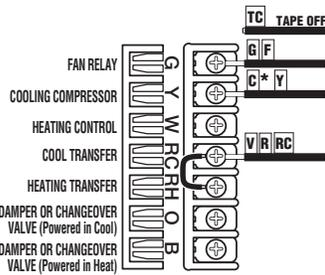
\* If both "Y" and "C" wire are present, tape off "C" wire.
