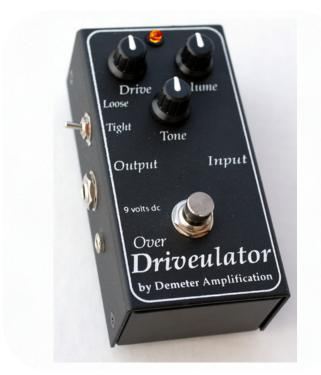
**Tight-Lose Switch**: This switches between Silicon and Germanium diodes for the distortion generating devices. Silicon Diodes have a tighter sound and are a bit louder. Germanium diodes have a looser more classic distortion sound with less output volume.
