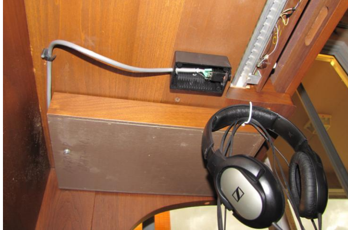
Photo #3a: Mounting the Jack Box underneath the key bed. In this photo the jack box cover is shown removed.
